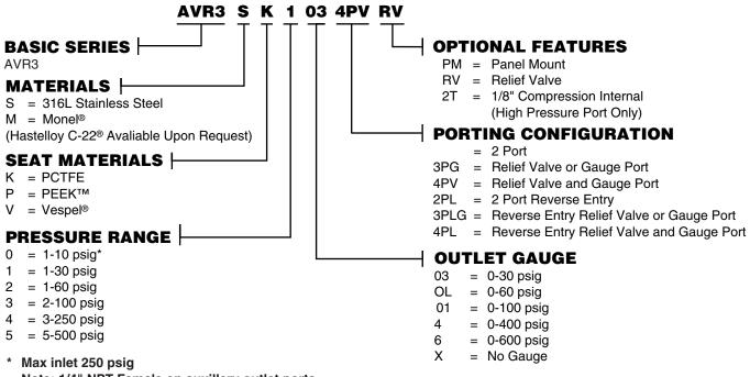
Note: 1/4" NPT Female on auxillery outlet ports. High Pressure port: 1/8" NPT Female is standard
