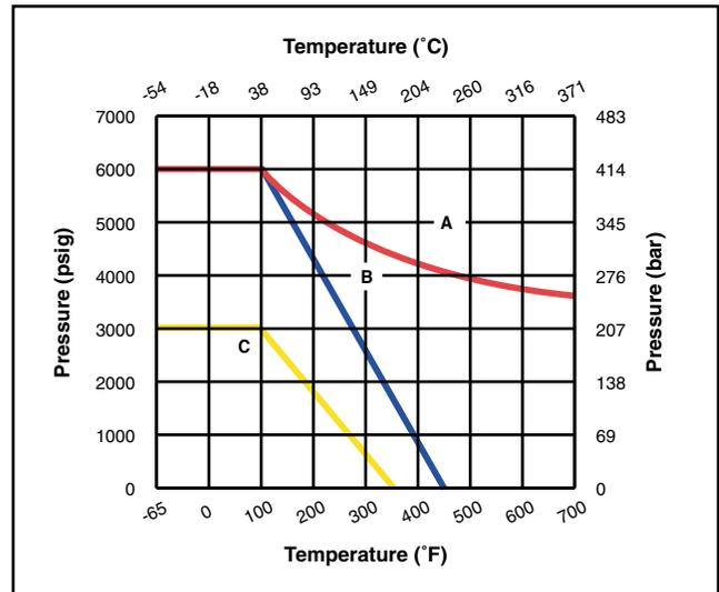
**Legend:** A - Grafoil® packing with R stem; B - PTFE packing with R stem; C - PTFE packing with K stem.
